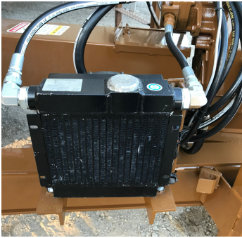
TWO SPEED COOLER
